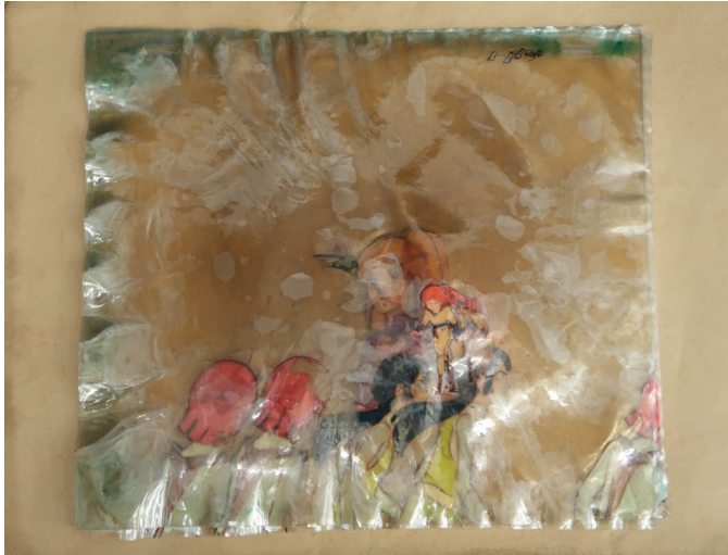
Examples of cels with severe vinegar syndrome damage.
