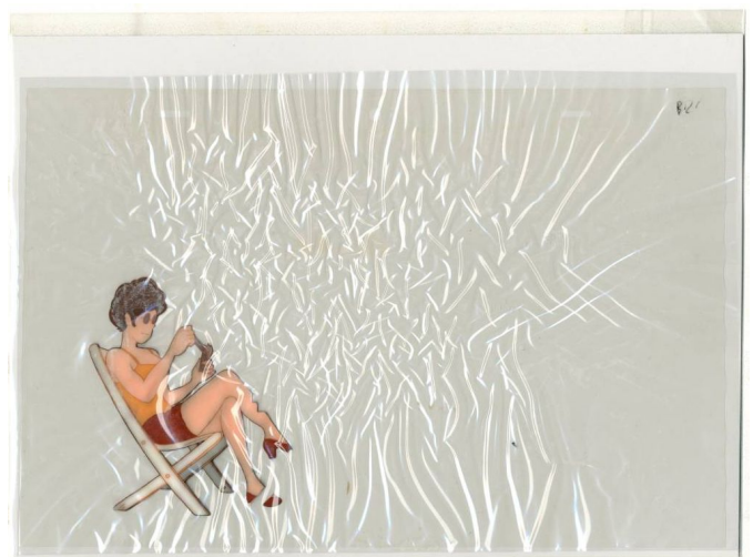
Examples of cel warping/rippling, indicative of vinegar syndrome.
