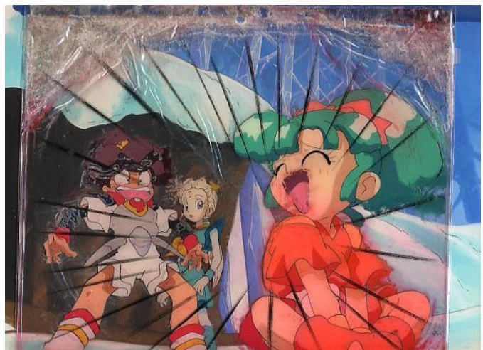
Examples of Vinegar Syndrome cels exhibiting grainy/crystal-like deposits. It is not known how to stop or remove this type of damage once it has occurred.
