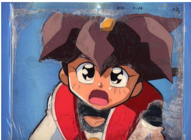
Examples of Vinegar Syndrome cels exhibiting grainy/crystal-like deposits. It is not known how to stop or remove this type of damage once it has occurred.
