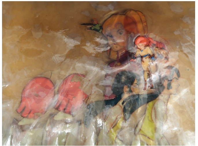
Examples of cels with severe vinegar syndrome damage.
